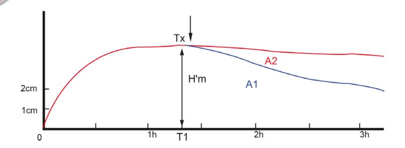
H'm: maximum height of the gas release curve.
