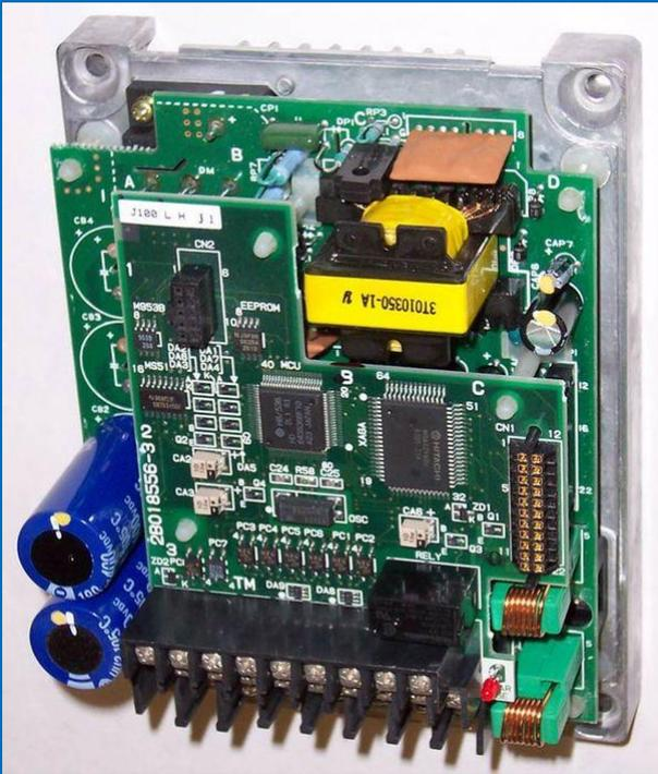
A **variable-frequency drive (VFD)** (also termed *adjustable-frequency drive*, *variable-speed drive*, *AC drive*, *micro drive* or *inverter drive*) is a type of adjustable speed drive used in electro mechanical drive systems to control AC motor speed and torque by varying motor input frequency and voltage .
