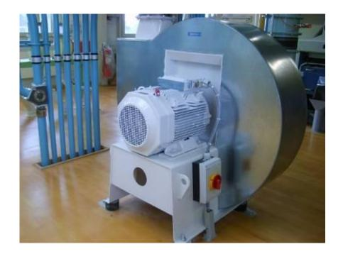
High pressure fan with frequency converter
