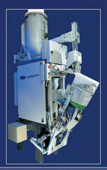
Valve packer for filling valve bags with using air pressure.
