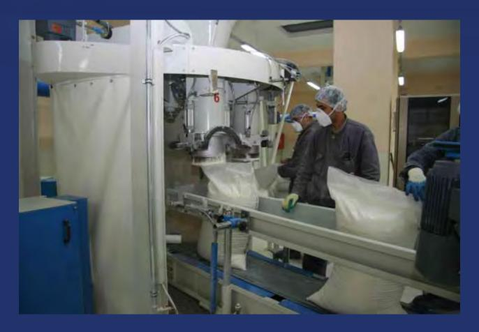
The bag is transferred in upright position into the bag closing device.
