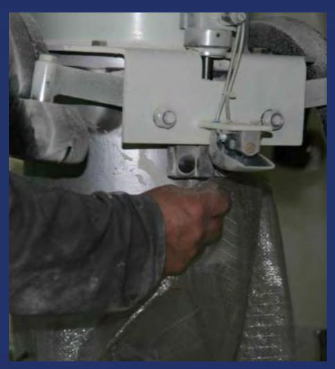
The empty bag is placed onto the spout.
