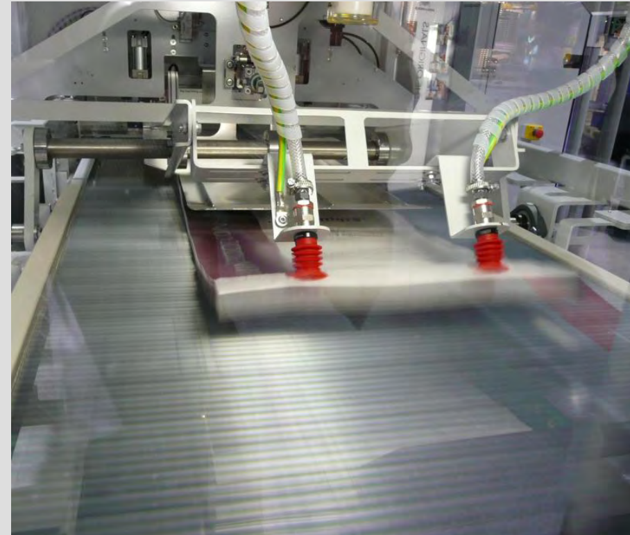
bag transport to the opening station
