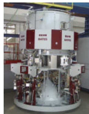
Rotoseal system according to the air filling principle – can be extended from 6 to 8 spouts
