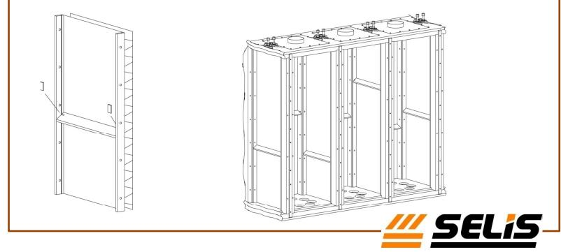
5- Diverting blocks ,made from aluminium profiles , can be fixed easly on any place along the passage
